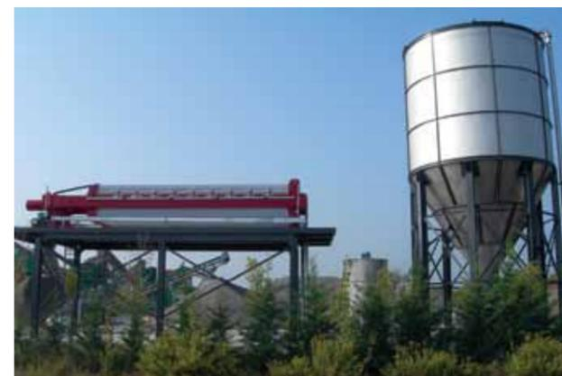
Filterpress and deep cone thickener tank
