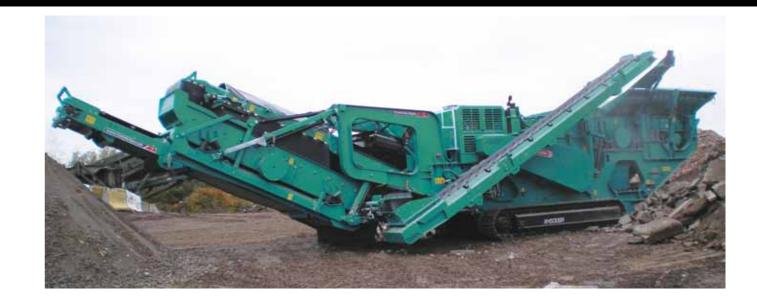
The Powerscreen® XH500 is the flagship horizontal shaft impactor. It is versatile, efficient and highly productive, offering both excellent reduction and a high consistency of product yield in quarrying, recycling and demolition applications. It is ideally suited to contract crushing due to its high productivity and ease of set-up, operation and maintenance.
