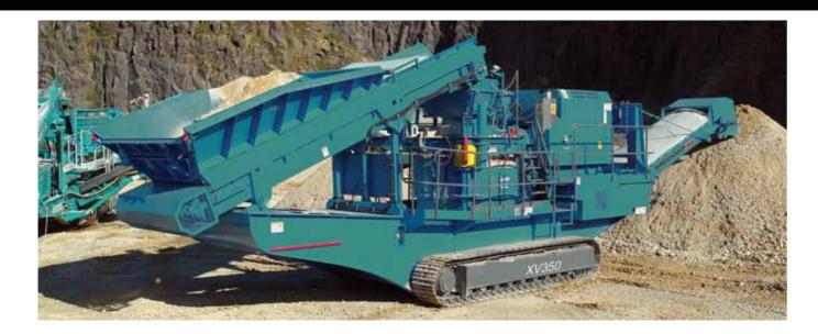
The Powerscreen® XV350 vertical shaft impactor is designed for users requiring a plant that excels at producing high specification, shaped products.
