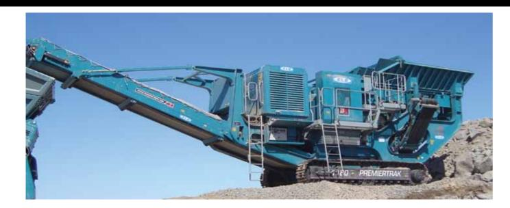
The Powerscreen® 1180 Premiertrak is a medium to large scale mobile primary jaw crusher plant which achieves high outputs in a variety of quarrying, recycling and contract crushing applications. The crusher features a high swing jaw with a forceful motion that improves feed entry into the crushing chamber to maximise throughput and allow for excellent reduction. User benefits include low fuel consumption, track mobility and simplified set-up, operation and maintenance.
