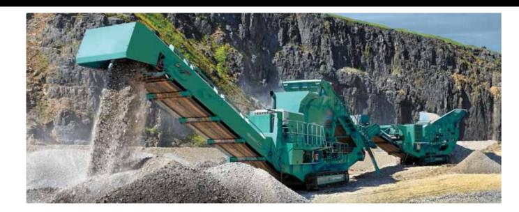
The Powerscreen® 1500 Maxtrak is one of the largest mobile cone crushers on the market. Specifically developed for larger users, the plant can accept an all in feed from a primary crusher to produce large volumes of aggregate.
