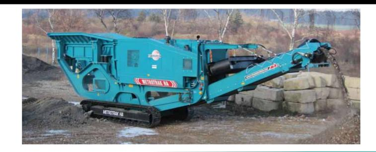
The Powerscreen® Metrotrak is a compact, high performance track mobile jaw crushing plant. With an aggressive crushing action and a high output even at tight settings, the Metrotrak is ideally suited for small to medium sized operators in the mining, quarrying and recycling industries.
