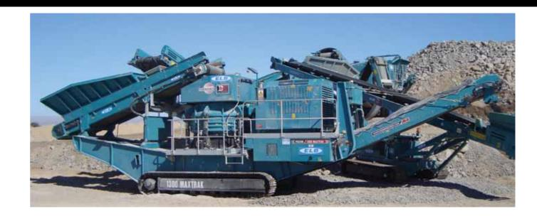
The Powerscreen® 1300 Maxtrak is a medium to large sized track mobile cone crusher which is ideally suited to secondary applications such as taking an all in feed from a primary crusher. Based around the 1300 Automax® cone crusher, the plant excels in the production of sub-base or aggregates, providing excellent cubicity, throughput and reduction ratios.
